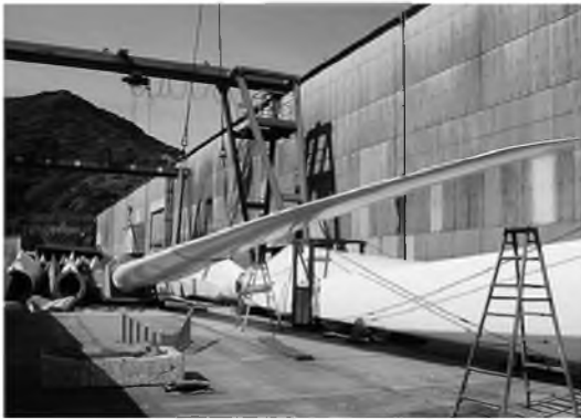
Fig. 16 Maximum load test of 36 m blade for 2 000 kW
