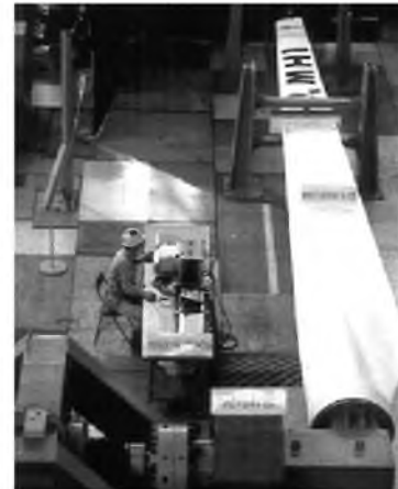
Fig. 7 Fatigue test of 29.5 m blade
