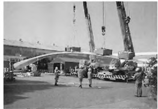
Fig. 6 Maximum load test of 29.5 m blade
